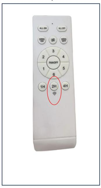
Point the remote at the fan. Hold the 2H button for 3 seconds.
